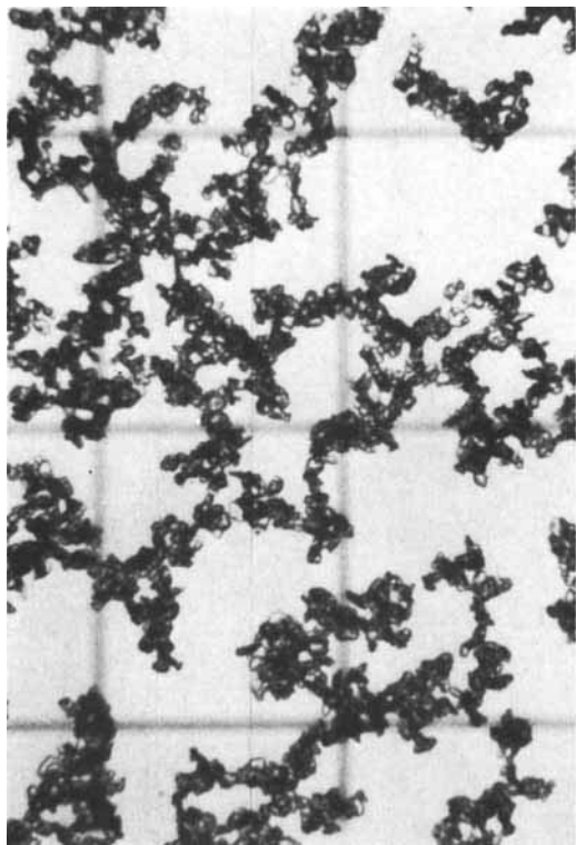
Fig. 11.—Photomicrograph of the suspension completely flocculated with the required concentration of McIlvaine buffer. The width of each scale division equals 96 \mu .
